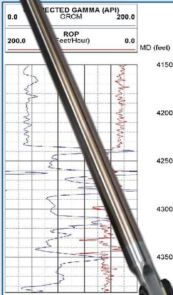
APS's next-generation SureShot natural gamma sensor employs a rugged scintillation counter and photomultiplier mounted in a specially designed package which provides protection against the high levels of shock and vibration encountered in the drilling environment. In addition, this extensively qualified new design offers environmental monitoring capability and lower power consumption, while maintaining back-compatibility with APS's earlier sensor designs.
