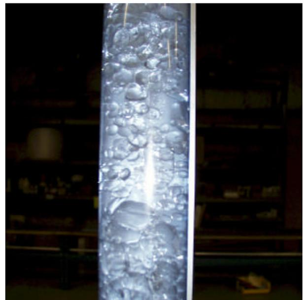
**Fig. 16: Example of flow pattern observed in test section while in vertical orientation; oil droplets suspended in water.**
