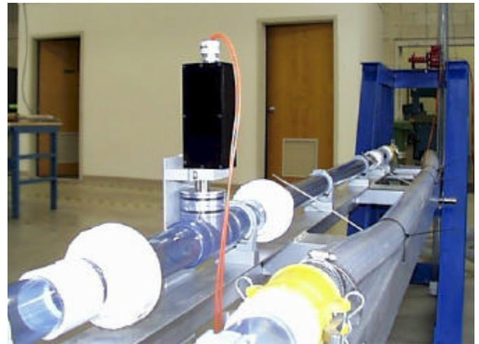
**Fig. 15: Movable section of flow loop showing fluorescence test fixture.**
